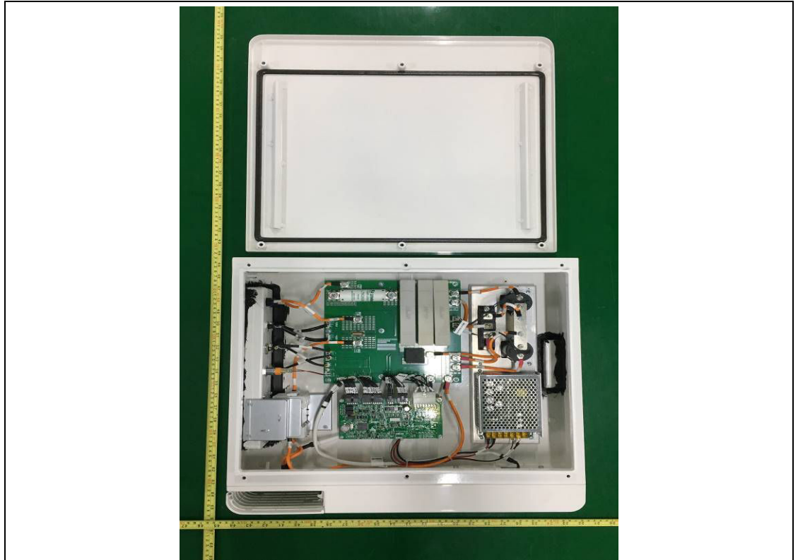
Internal view-1 of power control module
