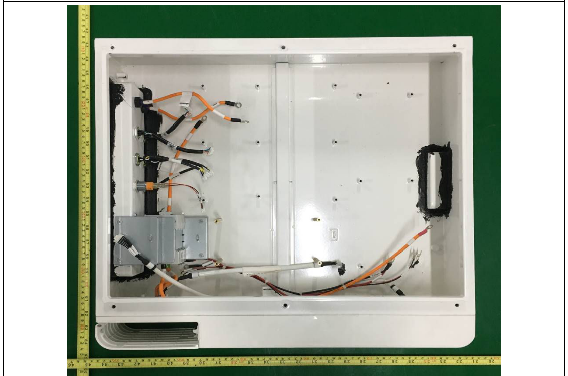
Internal view-2 of power control module
